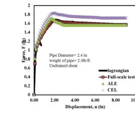
Figure Axial Force Displacement Responses for Pipe Sliding on Soil with Undrained Shear Strength of 0.03 kPa.
