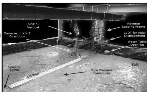
Figure Axial Pipe Soil Interaction Testing Facility at CIGMAT (Center for Innovative Grouting Materials and Technology)
