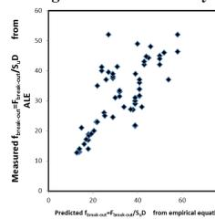
Figure Comparison of the Breakout Resistance Calculated from Empirical Equation and from ALE Finite Element Analyses
