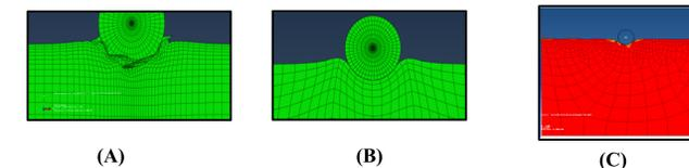
Figure Numerical Analysis: (A) Pure Lagrangian, (B) ALE, and (C) CEL
